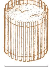
A simple bin of snow fencing is constructed by crimping the wire ends together to form a hoop.
